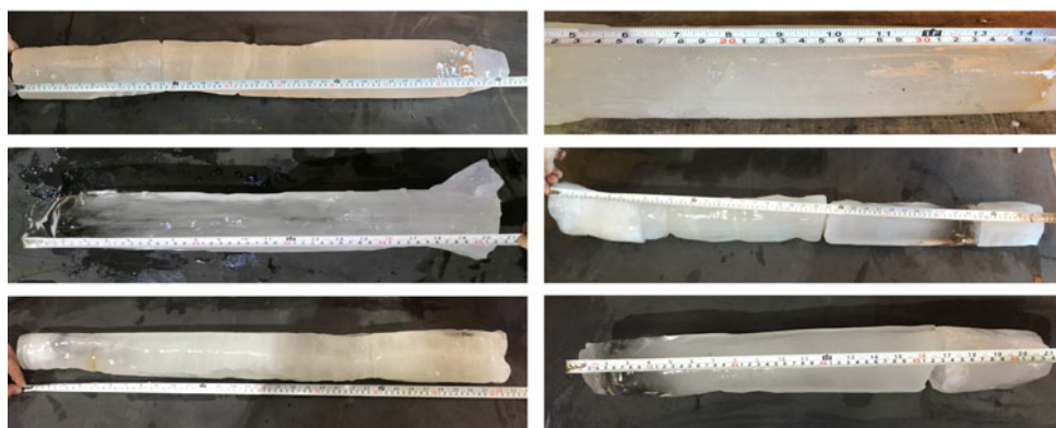
Fig. 7. Ice cores retrieved by the hot-water ice-coring drill.
