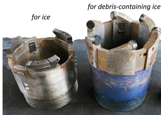
Fig. 6. Two types of drill bits used in ice drilling.
