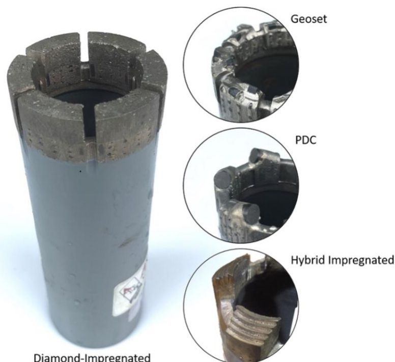
Fig. S1. Winkie Drill is equipped with four bit designs. The #10 diamond-impregnated bit is used in hard bedrock formations. The geoset bit is used in soft rock formations or when sediments are entrained in the ice. The polycrystalline diamond compact (PDC) bit can be used in similarly soft rock formations but has had limited success when ice is present in the kerf. The hybrid impregnated bit is made from the same material as the standard #10 diamond-impregnated bit but includes a relief angle behind the leading edge. This bit can cut ice and transition into bedrock. Figure reproduced from Boeckmann and others, 2020; Fig. 4.
