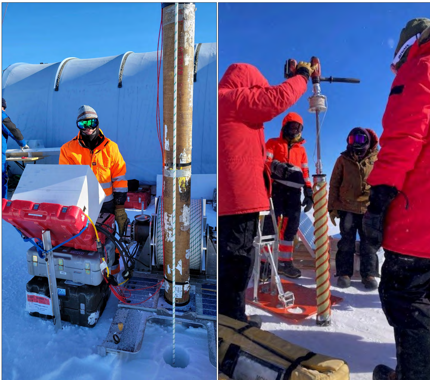
(Left) IDP Engineer Jay Johnson operates the 4-Inch Drill outdoors and behind wind screens at Dome C. Credit: Estelle Vincent.
